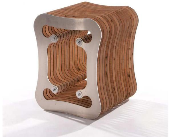
The Diviso Stool is made using only two manufacturing processes and with flat pack capability for ease of delivery to buyers across the world. Each of the stool's profiles are precision laser cut and spaced with acrylic which also houses four aluminium supports. The stool is lightweight and can easily support up to 120kg. The stool is a completely concentric shape, creating a beautifully proportioned piece of furniture.
